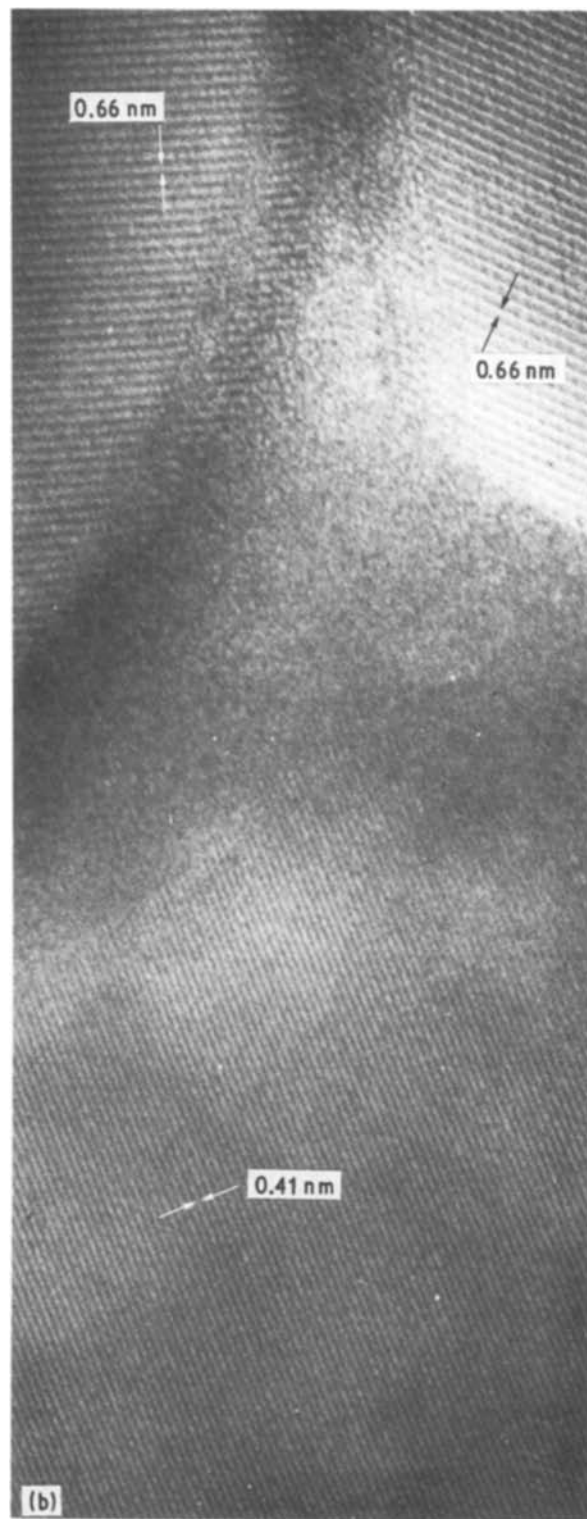
Figure 6 Lattice images showing the presence of intergranular films in the central region of Fig. 5. (a) Intergranular film between the \beta -grains 1 and 2 (see Fig. 5a). The lattice fringes correspond to \{10\bar{1}0\} planes (spacing 0.66 nm) in both grains. Grain 1 has an orientation which is close to an [0001] beam direction giving rise to the two sets of lattice fringes visible in this grain. (b) Intergranular film in the vicinity of the triple junction between \beta - \text{Si}_3\text{N}_4 grains 1 and 2 and the Y,N-apatite grain. The lattice fringes in the Y,N-apatite grain correspond to the \{200\} planes with a spacing of 0.41 nm.
